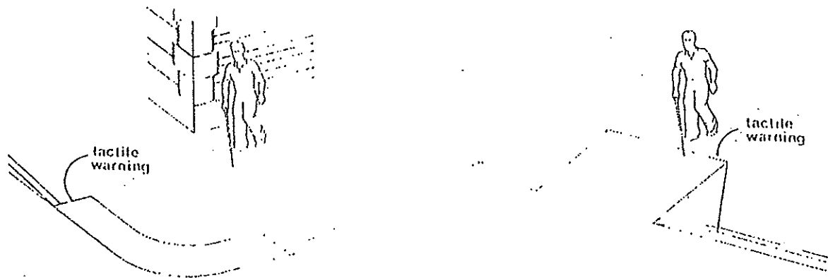
Fig. 14 Warning Signals at Curb Ramps.
